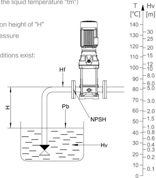
**NOTE:** To avoid cavitation, the pump should be rated away from the right side of the NPSH curve. Always check the NPSH value of the pump at the highest possible flow.
